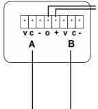
The **GS-42** provides a 5V or 12V sensor supply (the selected sensor voltage is present only during transmission or if the sensor supply is enabled in TxSetup).
