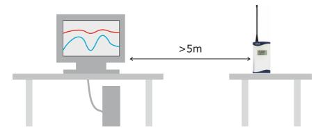
If the Receiver is connected directly to the PC, an RS232 extension lead may be required (RS232/5M for 5m). Alternatively, use an external antenna on the Receiver if installation permits:
