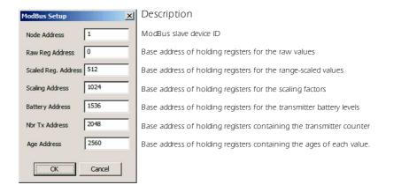
When reading the values from the RC250, the only Function Code that can be used is 'Read Holding Registers' (0x03). It is possible to read several registers at a time using the Quantity of Registers field, but note that RC250 is limited to 50 registers at a time.
