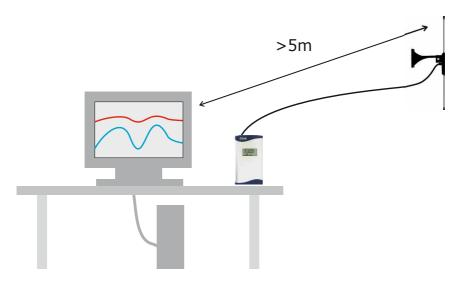
The Receiver should also be located clear of all other sources of radio interference.
