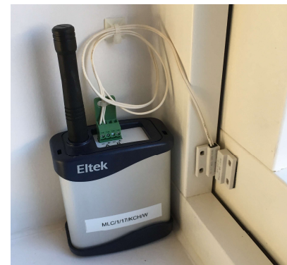
Wirelessly monitoring how often windows are opened and closed.
